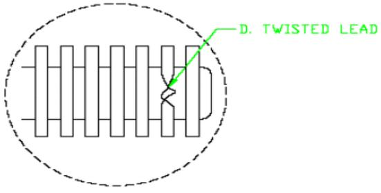
A schematic diagram of a terminal lead assembly. A dashed circle highlights a lead that is twisted. A green arrow points to this lead with the label "D. TWISTED LEAD". |
