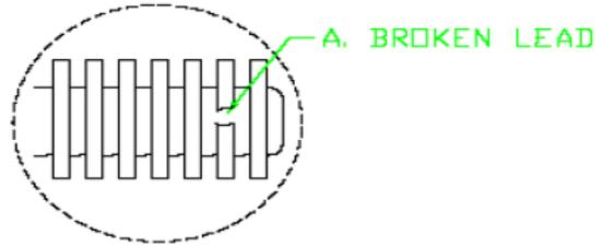
A schematic diagram of a terminal lead assembly. A dashed circle highlights a lead that is broken. A green arrow points to this lead with the label "A. BROKEN LEAD".   |
