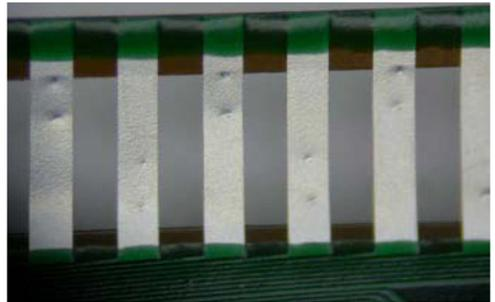
A photograph showing a row of terminal leads. Each lead has a small, dark, rectangular mark on its top surface, which are the prober marks.                                              |
