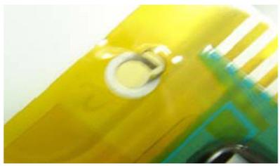
A close-up photograph of a yellow printed circuit board (PCB) showing a circular hole in the copper film, exposing the underlying substrate.                                              |
